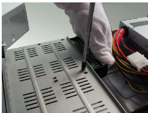
2. Mount the hard drive on the rack.
