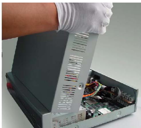
4. Put back the cover after hard drive(s) installed. Note: plug the front part of the cover into the slot on the box and then push down the cover.
